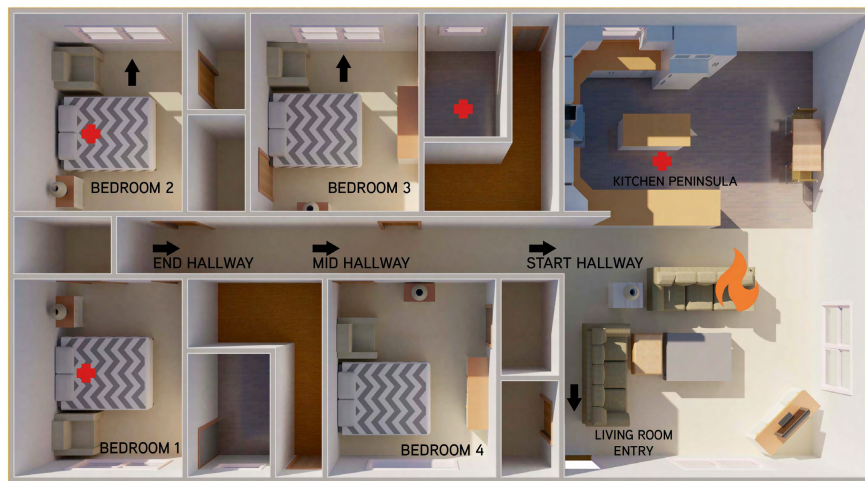
Figure 6.5: Toxic gas exposure measurement locations. The red plus signs are locations of potentially trapped occupants and the black arrows are measurement locations along potential egress pathways.
