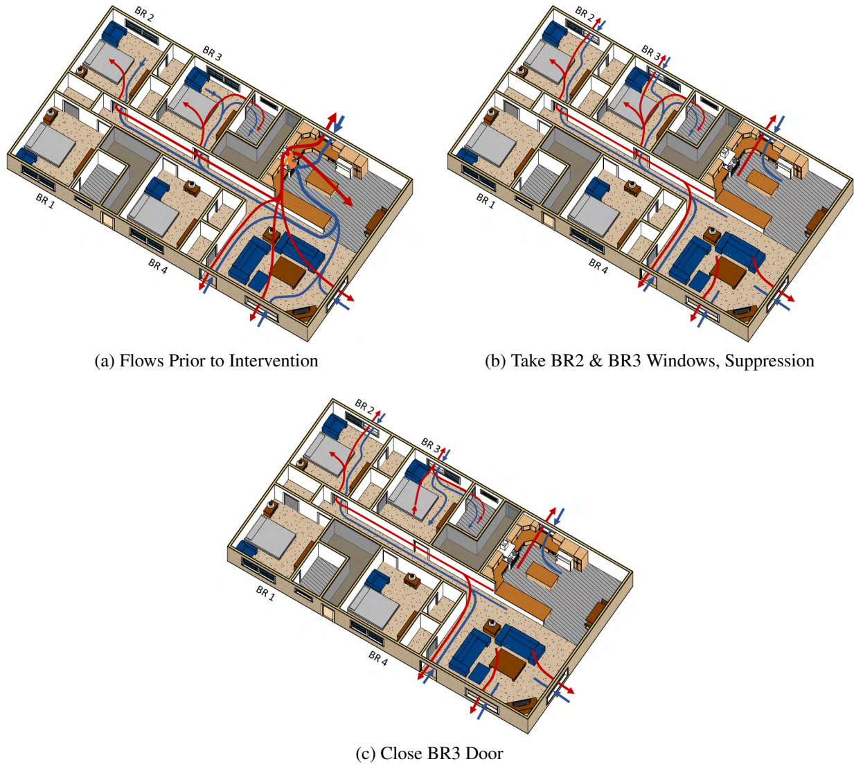
Figure 5.15: Changes in gas flows within the structure following fire department interventions in Experiment 12.
