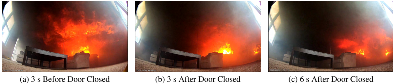
Figure 5.79: Fire conditions preceding and following front door closure during Experiment 16.
