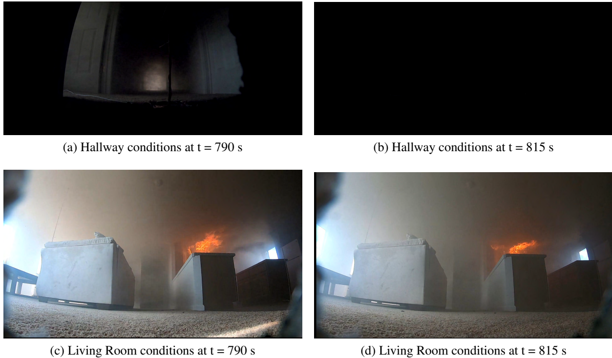
Figure 4.13: Loss of visibility at hallway camera location compared to living room camera location during Experiment 18.
