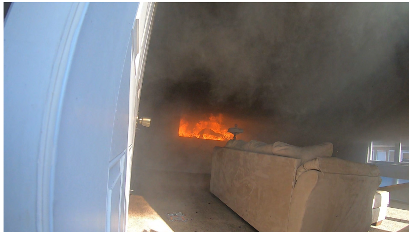
Figure 5.96: Fire conditions immediately prior to search crew entering structure during Experiment 17.
