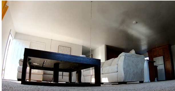
(a) Initial Ceiling Temperature Rise (40 s)
