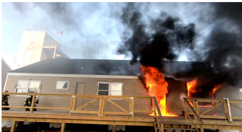
Figure 4.26: Side A exterior image of conditions at the front door and living room windows prior to first firefighter intervention for a living room fire (Experiment 19).
