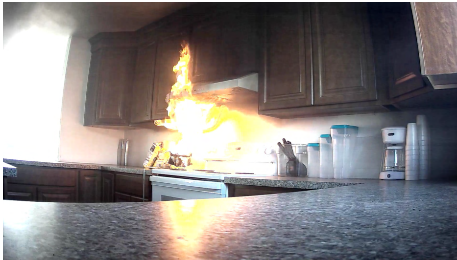
Figure 4.3: Camera view of fire beginning to spread from oil pan to kitchen cabinets at t = 406 s.
