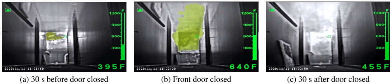
Figure 5.81: Hallway IR view in period preceding and following front door closure in Experiment 16.
