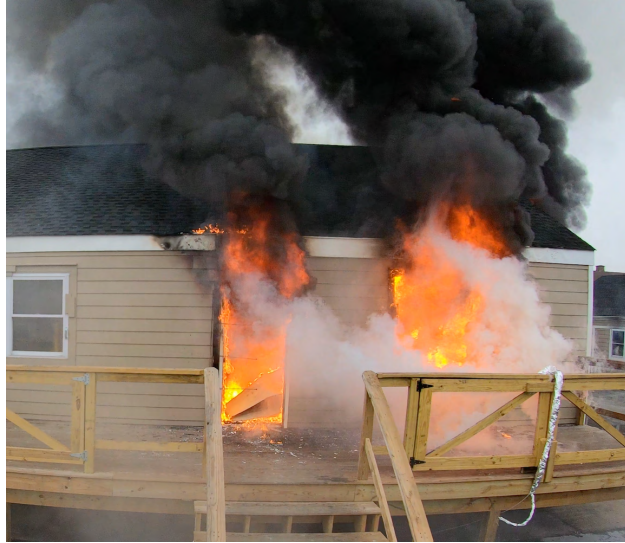
Figure 5.38: Photograph of front door panel fold over prior to suppression.
