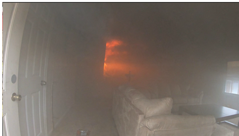
Figure 5.63: Fire conditions immediately prior to front door closing during Experiment 15.
