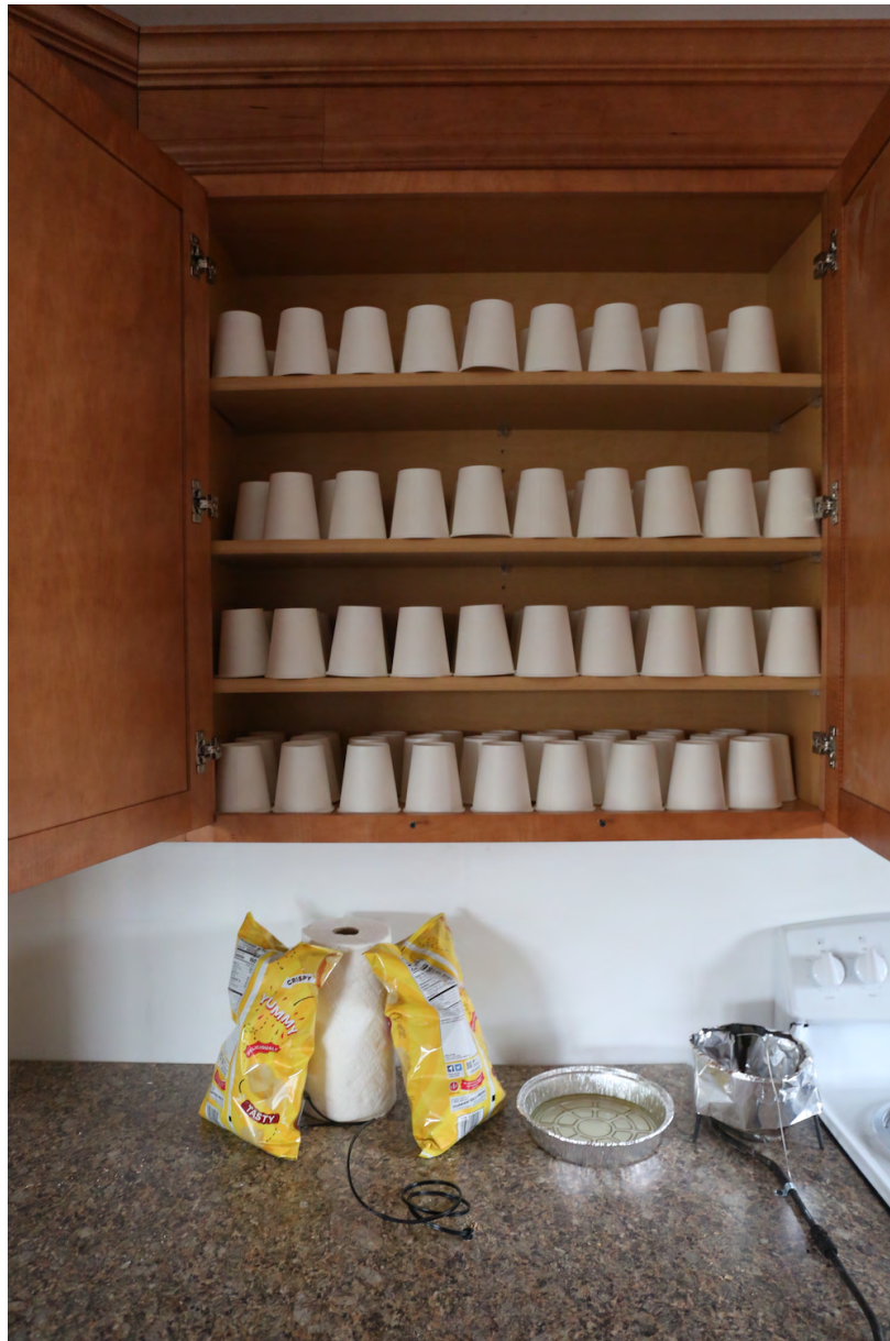
Figure 3.10: Photograph of ignition setup for kitchen fire. Prior to ignition of the pilot burner, the cabinet doors were closed. The pan of oil was placed on top of the stand above the burner after the burner is ignited.
