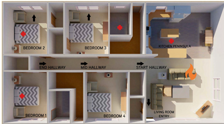
Figure 6.7: Thermal exposure measurement locations. The red plus signs are locations of potentially trapped occupants and the black arrows are measurement locations along potential egress pathways.
