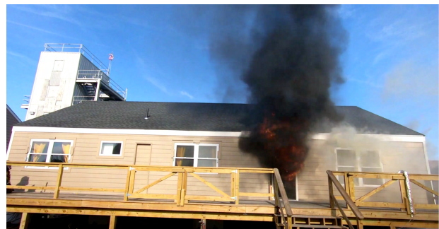
(b) Side A Exterior At First Visible Exterior Flames (238 s)
