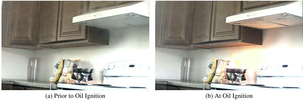
Figure 4.1: Still images from kitchen ignition video prior to and at ignition of cooking oil on kitchen counter.
