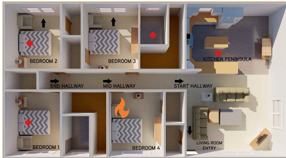
Figure 6.5: Thermal exposure measurement locations. The red plus signs are locations of potentially trapped occupants and the black arrows are measurement locations along potential egress pathways.
