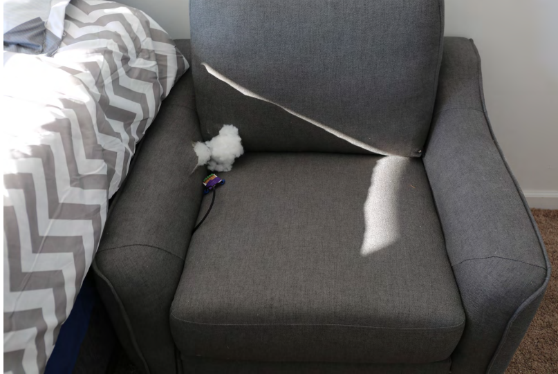
Figure 3.8: Photograph of ignition setup for a bedroom fire.
