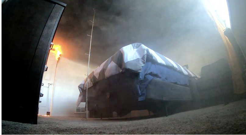
Figure 5.135: Pre-intervention Bedroom 3 Door Combustion
