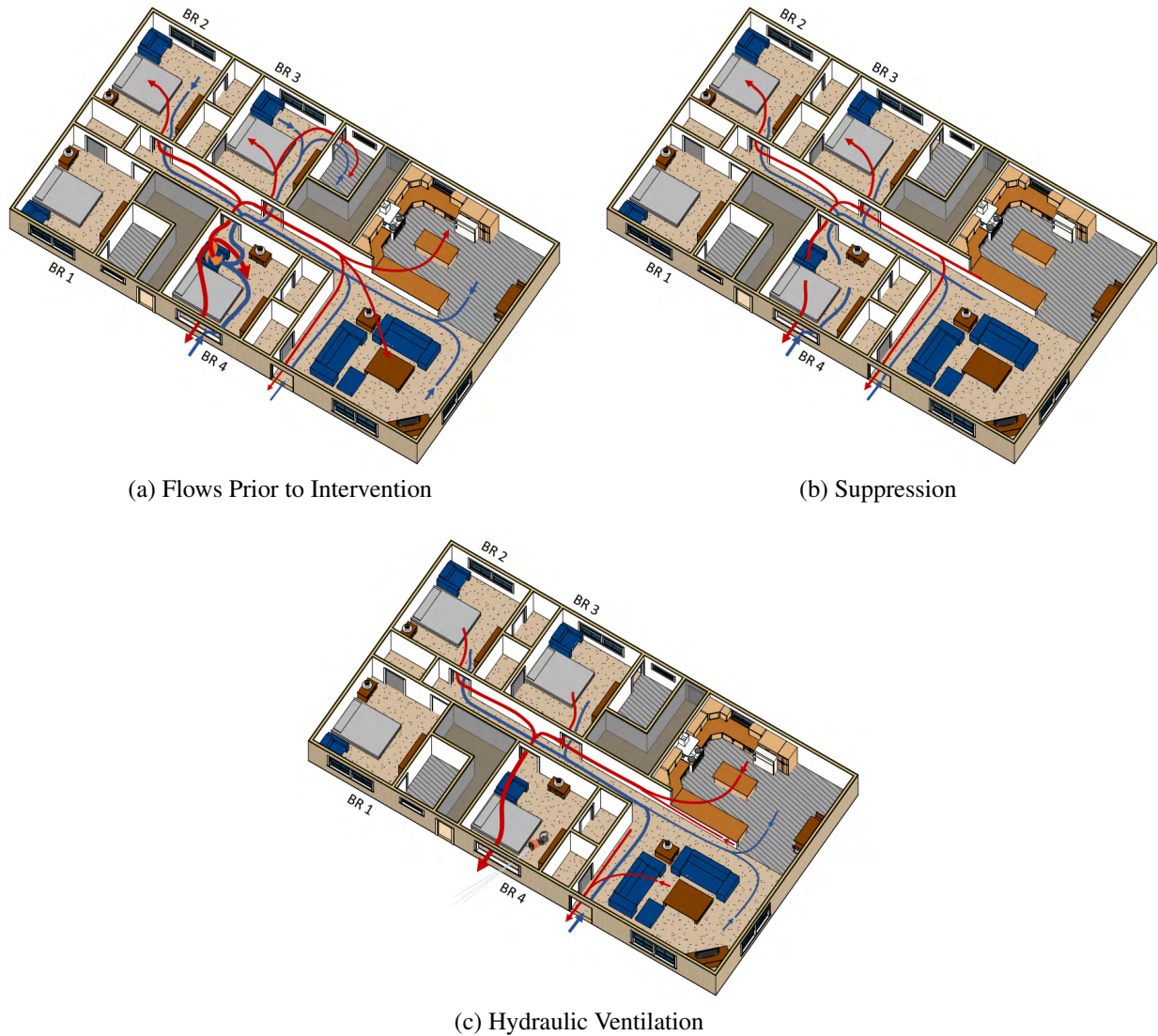
Figure 5.163: Changes in flow in structure following fire department interventions in Experiment 10.
