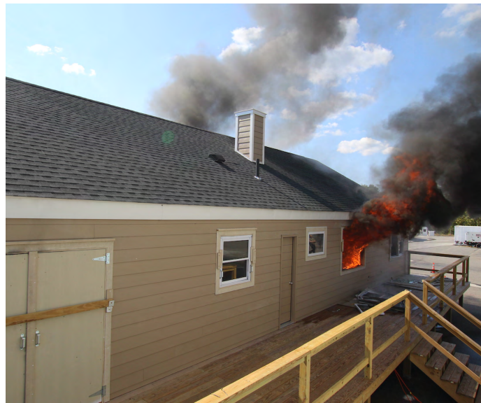
Figure 6.11: Photograph of side C exterior fire conditions at bedroom 3 window 90 s after window ventilation during Experiment 4.
