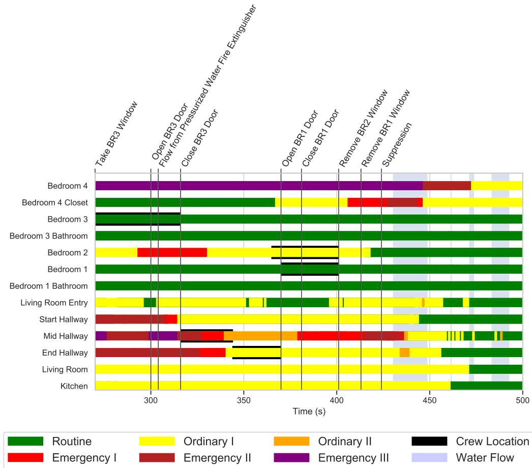
Figure 6.13: Comparison of thermal operating conditions based upon 3 ft elevation temperatures and heat fluxes during post-intervention period for pre-suppression window initiated search tactics into an isolated room (Experiment 8b).
