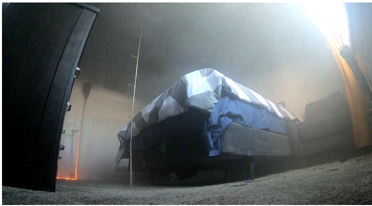
(b) Immediately Prior to Hallway Door Open (30 s Post Window Ventilation)
