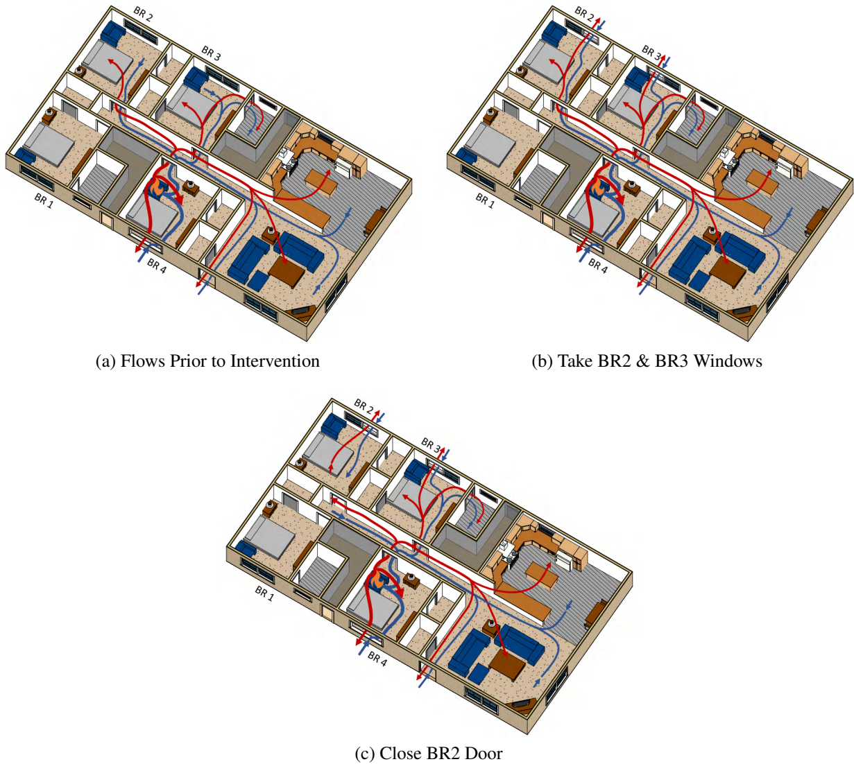
Figure 5.49: Changes in flow in structure following fire department interventions in Experiment 4.
