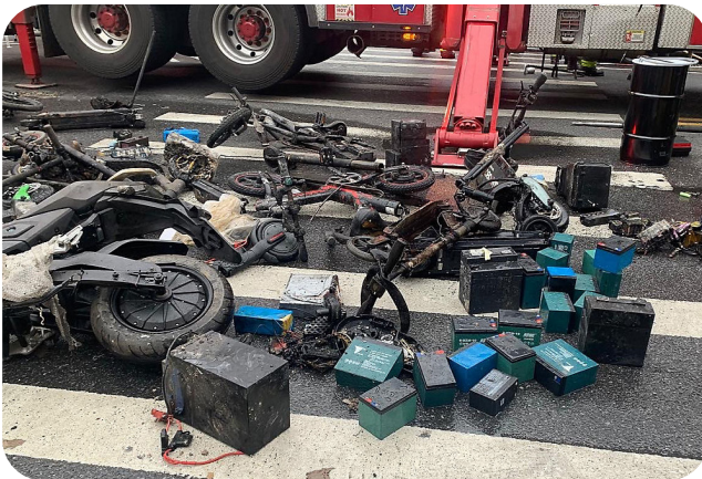
Lithium-ion batteries from e-mobility devices which caused a fire (FDNY)
