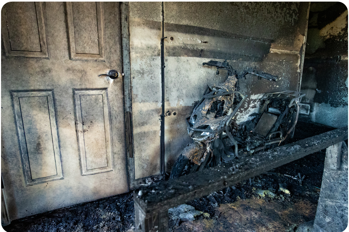
E-mobility device went into thermal runaway and caused a fire (FSRI)
