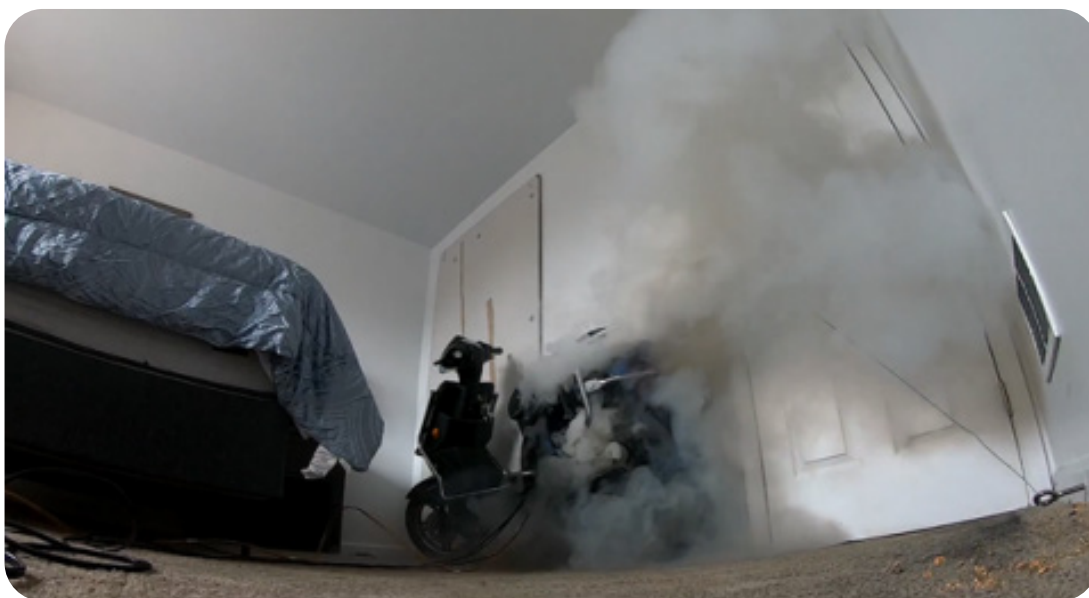
Smoke from e-mobility device, signifying the battery is in thermal runaway (FSRI)
