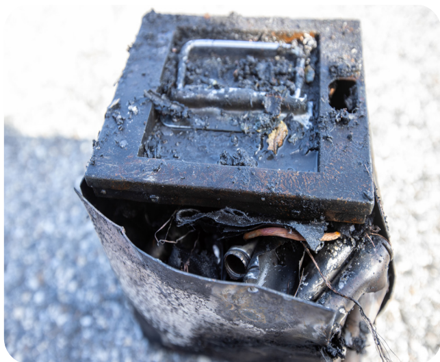
Lithium-ion battery post thermal runaway (FSRI)
