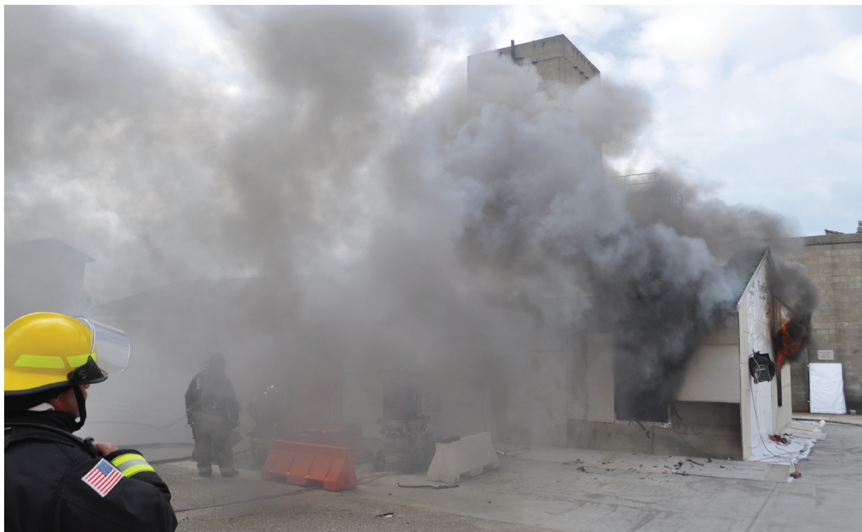
Fireground concentrations of benzene, total PAHs, and particulate were highest when collected downwind of the structure and when ground-level smoke was heaviest.
