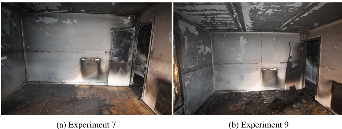
Figure 6.45: Post-furniture comparison of bedroom 1 wall opposite area of origin with closed door and windows.
