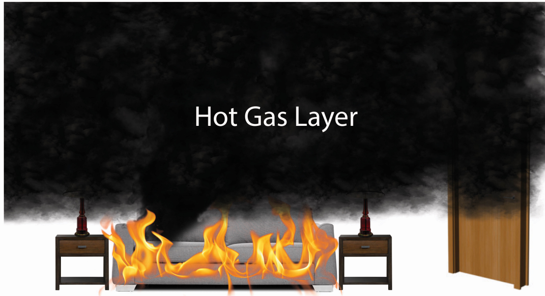
Figure 1.5: Drawing of the hot gas layer in a compartment fire.
