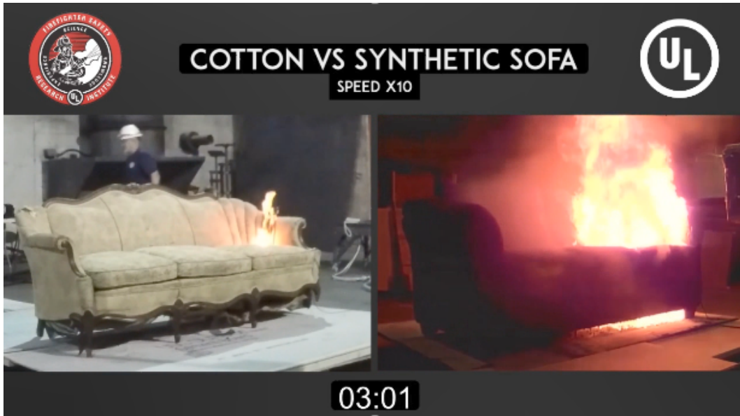
Figure 1.1: Comparison of upholstered sofas: cotton versus polyurethane foam. Images recorded approximately 180 seconds after ignition.
