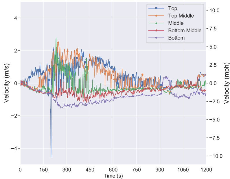
Figure 4.59: Experiment 7, no exterior ventilation openings, hallway velocity versus time. Positive velocity flowing from bedroom to living room.
