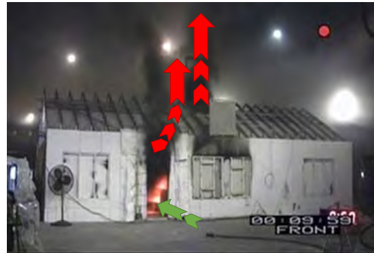
(b) Flow with Vertical Ventilation
