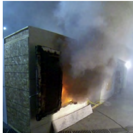
(b) Exhaust With Fan Flow - Pre Flashover
