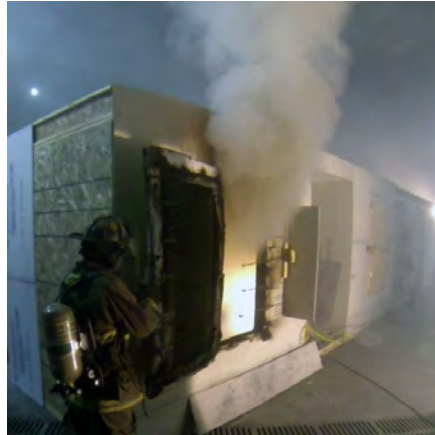
(a) Exhaust Without Fan Flow - Pre Flashover
