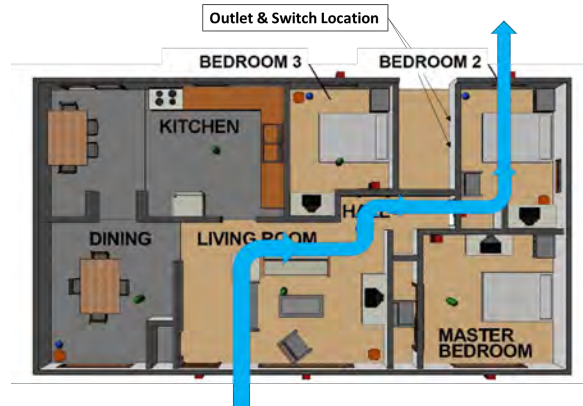
(b) Outlet and Switch Locations
