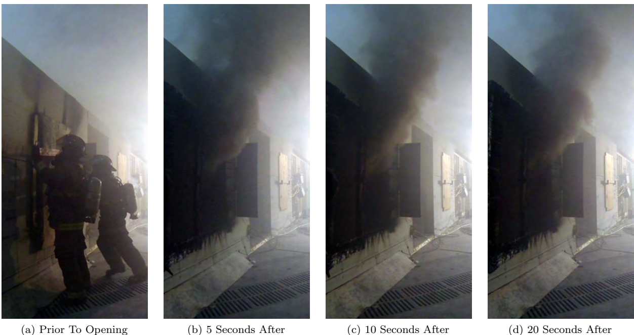
Figure 6.25: Non Fire Room Neutral Plane
