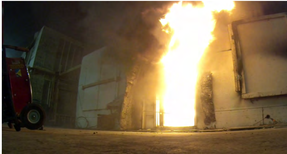
Figure 6.14: Vent Point Ignition of Fan Inlet During Laboratory Experiments
