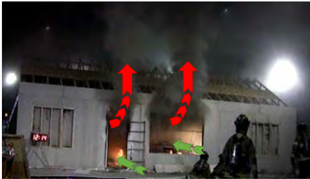
(a) Flow with Horizontal Ventilation
