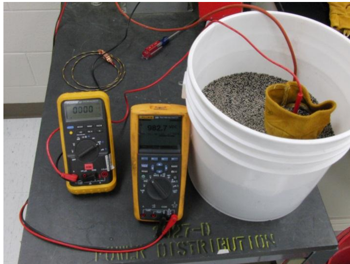
Figure 29 Testing a glove in metal shot
