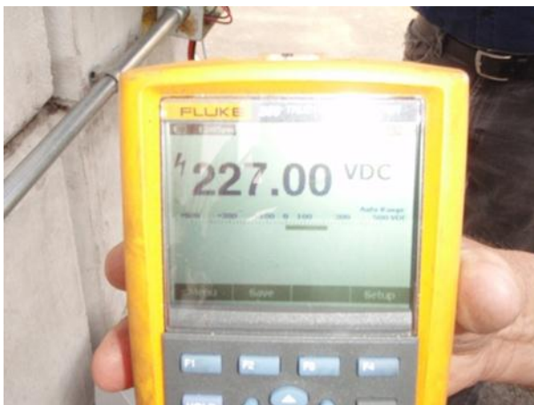
Figure 181 Installer identifies hazardous voltage Figure 182 Assessing Damaged Modules
