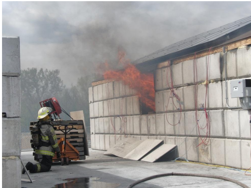
Figure 166 Fan used to help force flames towards roof
