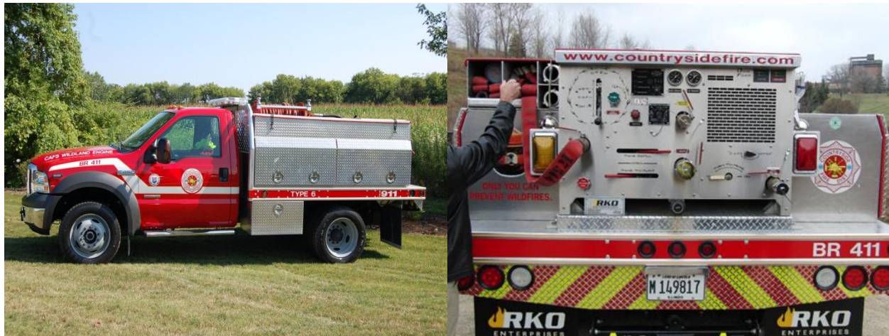
Figure 43 Fire truck with compressed air foam system
