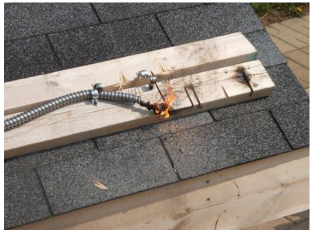
Figure 59 Open flame from arcing
