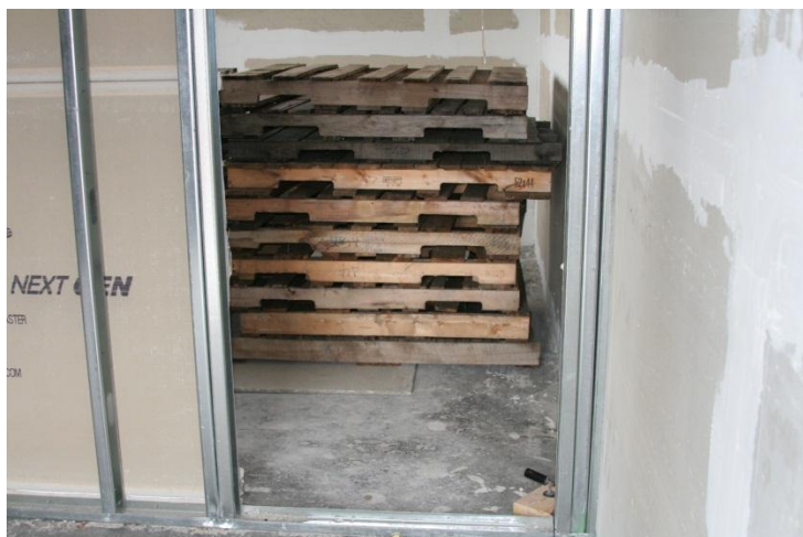
Figure 161 Photograph of wood skid fuel package in room.
