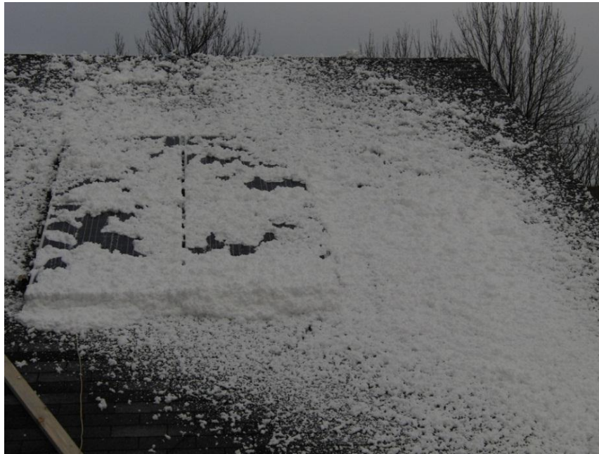
Figure 46 - After 10 minutes, gaps appearing in foam over modules
