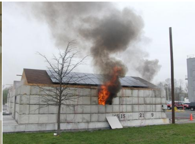
Figure 163 Flames forced out window opening
