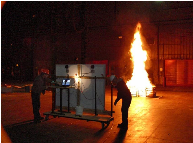
Figure 73 Test fixture with modules approaching fire
