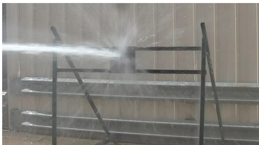
Figure 10 Water stream breaking up and dispersing near target plate
