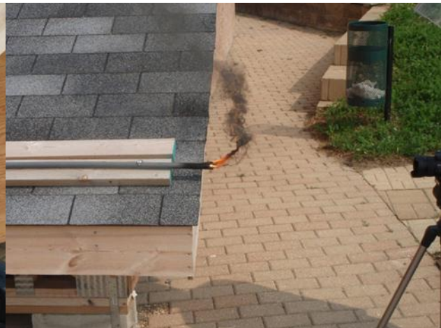
Figure 55 Open flame from arcing
