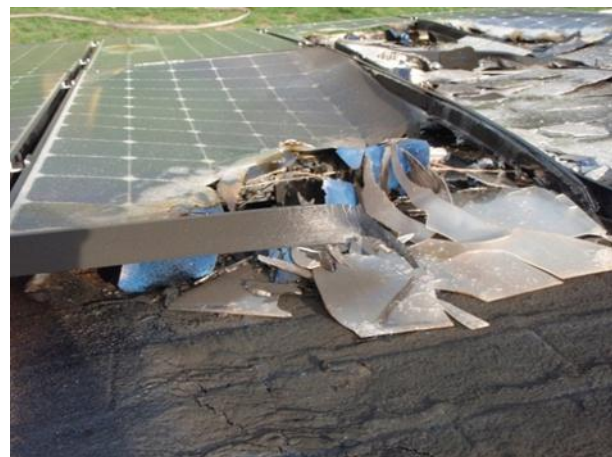
Figure 181 Installer identifies hazardous voltage Figure 182 Assessing Damaged Modules
