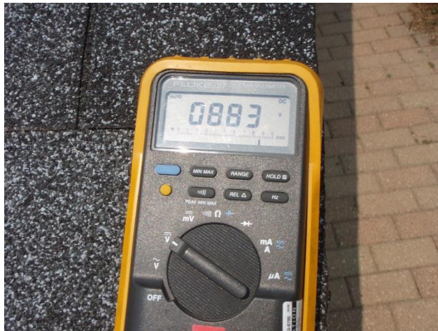
Figure 67 Voltage measured between metal pan and earth
