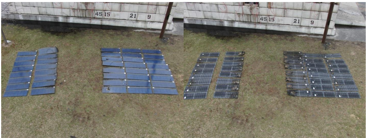
Figure 158 Array reconstructed on ground, post-fire
