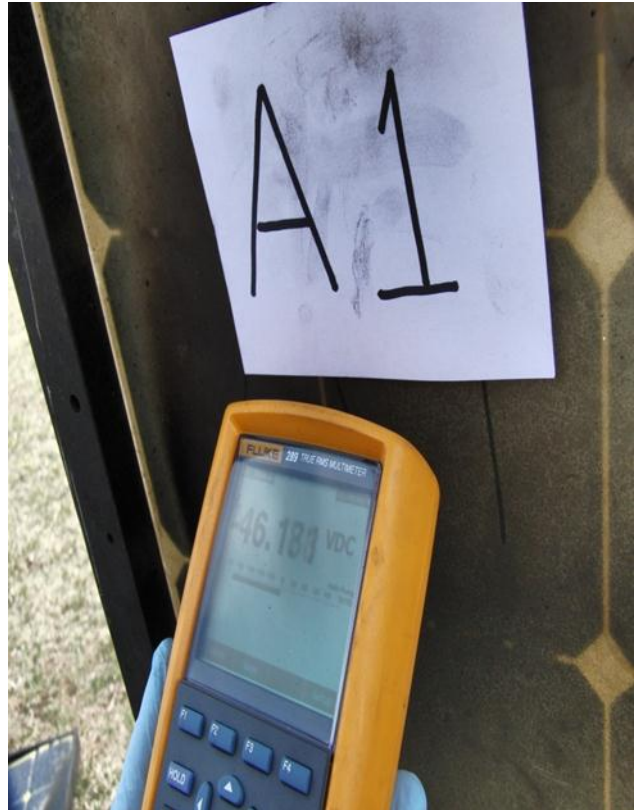
Figure 115 Module A1 – damaged but functional and producing full voltage
