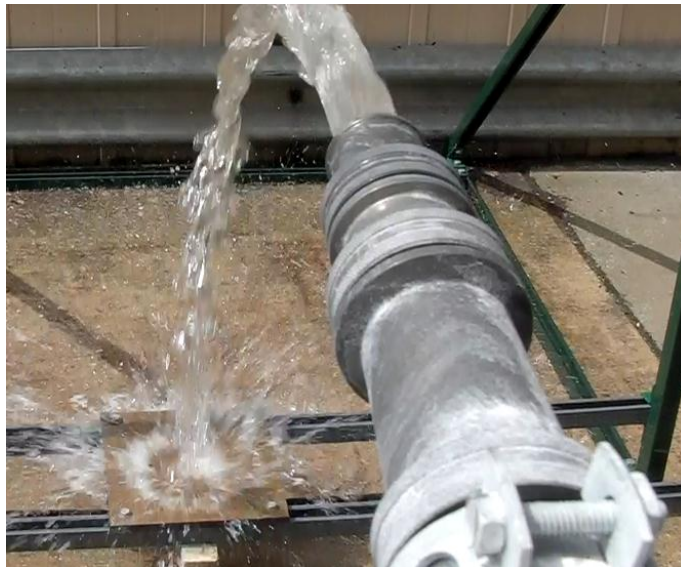
Figure 9 Water stream aimed at flat (horizontal) energized target plate
