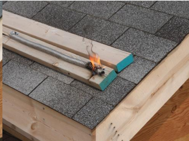
Figure 57 Open flame from arcing
