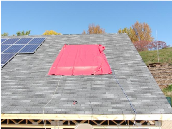
Tarp #4 – 12 x 14 foot heavy vinyl fire salvage tarp, red in color. Claimed to meet ASTM E-84 25 and UL 214 26 . Cost $94.
