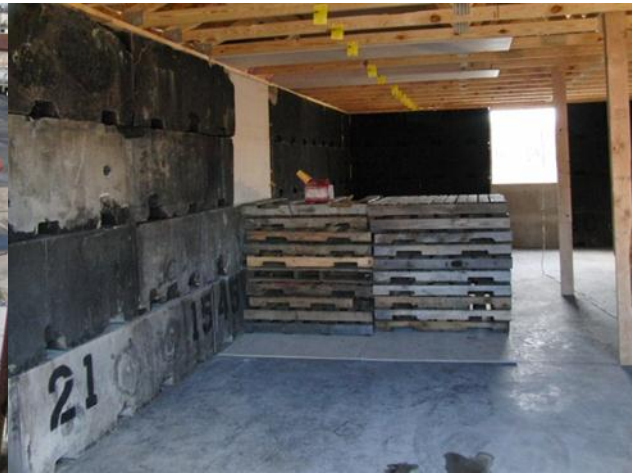
Figure 98 Wood pallets ready for ignition
