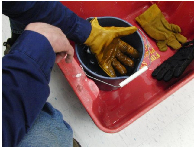
Figure 30 Wetting a glove before test
