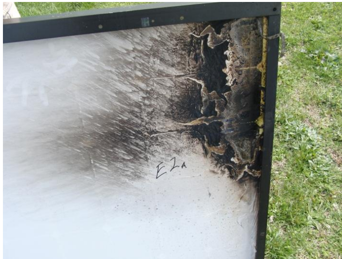
Figure 188 Module E2, partial damage
