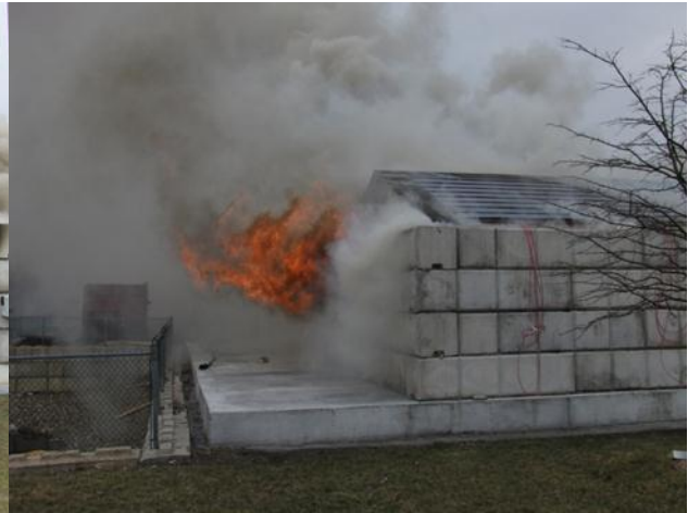
Figure 145 Flames from backside of roof
