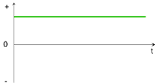
Figure 2. DC - peak voltage = DC (RMS) voltage
