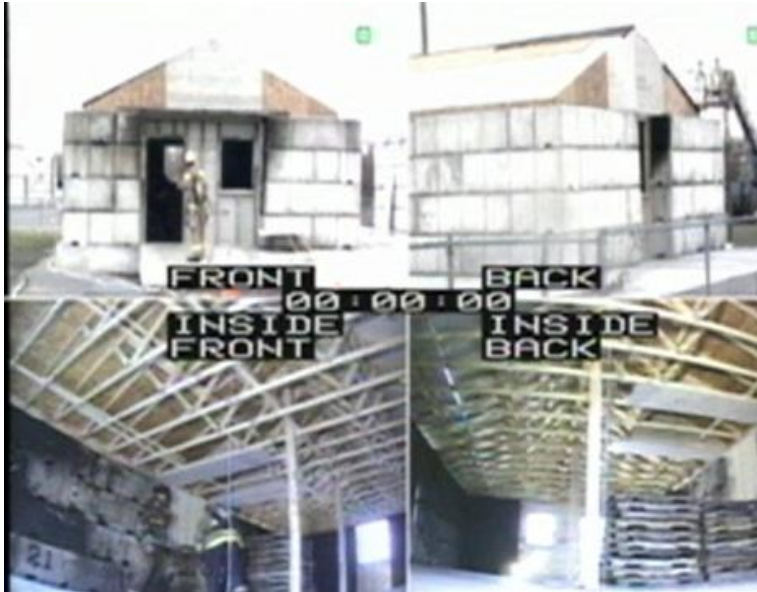
Figure 81 Quad Video 1 - Compartment / Roof Fire
