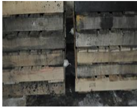
Figure 84 - Igniter In Wood Skids
