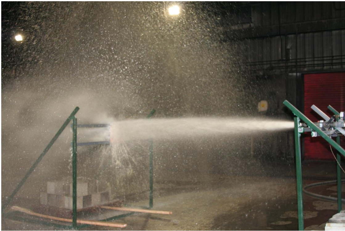
Figure 8 Water stream aimed at energized target plate
