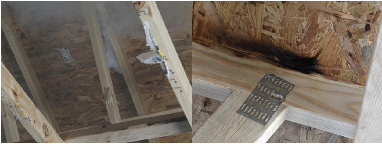
Figure 192 Smoke developing on inside of roof Figure 193 Charring on inside of roof
