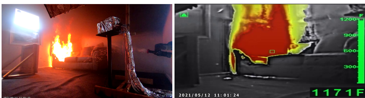
Figure 3.5: Standard and thermal imaging views of conditions in the fire room at start of suppression, 836 s (13:56) after ignition, in Experiment 1A.
