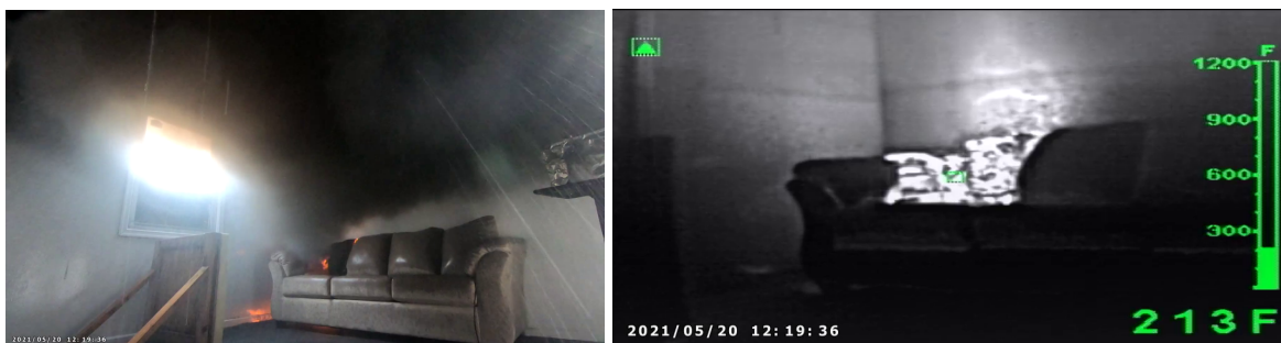
Figure 3.12: Standard and thermal imaging views of conditions in the fire room 30 s after nozzle activation (156 s (2:36) after ignition) in Experiment 5.
