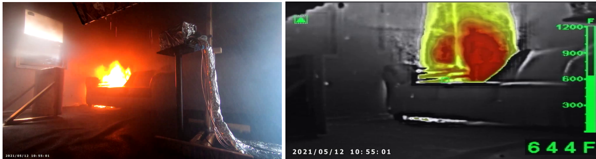
(a) Experiment 1A, 450 s (7:30) after ignition, 284 s (4:44) after water on
