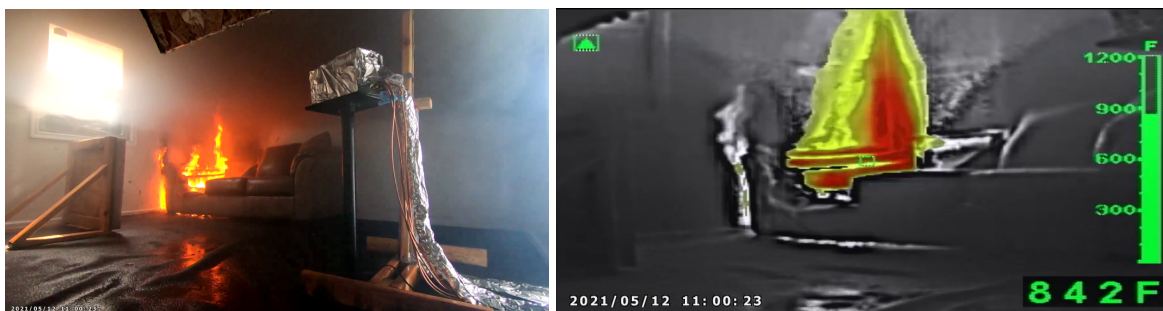
Figure 3.4: Standard and thermal imaging views of conditions in the fire room at end of water flow duration, 772 s (12:52) after ignition, in Experiment 1A.
