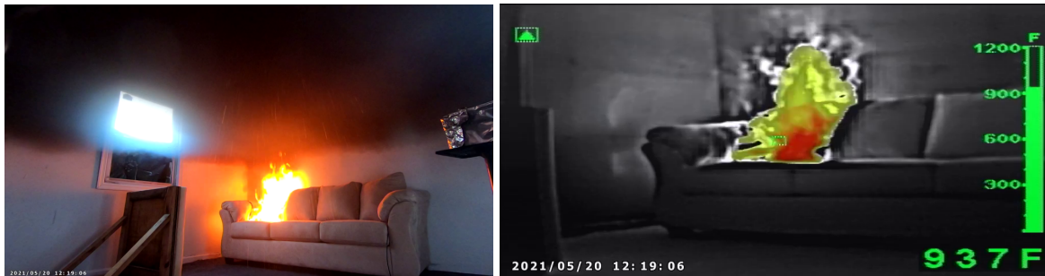
Figure 3.11: Standard and thermal imaging views of conditions in the fire room at nozzle activation, 126 s (2:06) after ignition, in Experiment 5.
