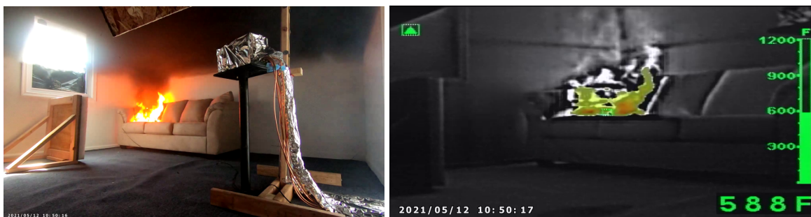
(a) Experiment 1A at nozzle activation, 166 s (2:46) after ignition
