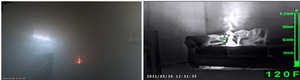
Figure 3.14: Standard and thermal imaging views of conditions in the fire room at start of suppression, 874 s (14:34) after ignition, in Experiment 5.
