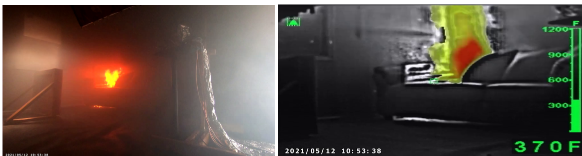
Figure 3.3: Standard and thermal imaging views of conditions in the fire room at time of hallway tell-tale sprinkler activation, 367 s (6:07) after ignition, in Experiment 1A.
