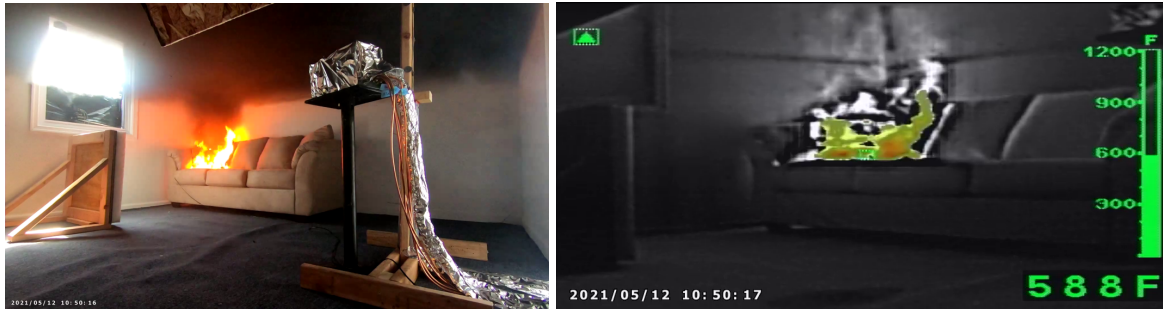
Figure 3.1: Standard and thermal imaging views of conditions in the fire room at nozzle activation, 166 s (2:46) after ignition, in Experiment 1A.
