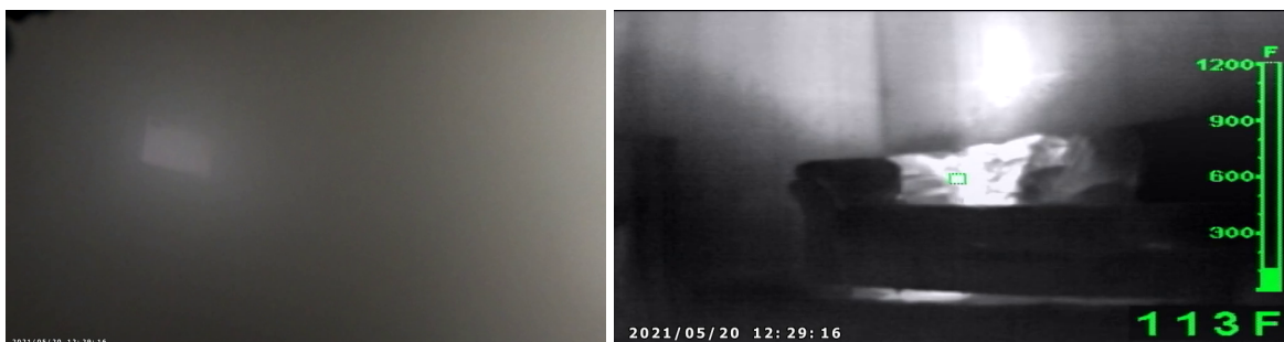
Figure 3.13: Standard and thermal imaging views of conditions in the fire room at end of water flow duration, 734 s (12:14) after ignition, in Experiment 5.
