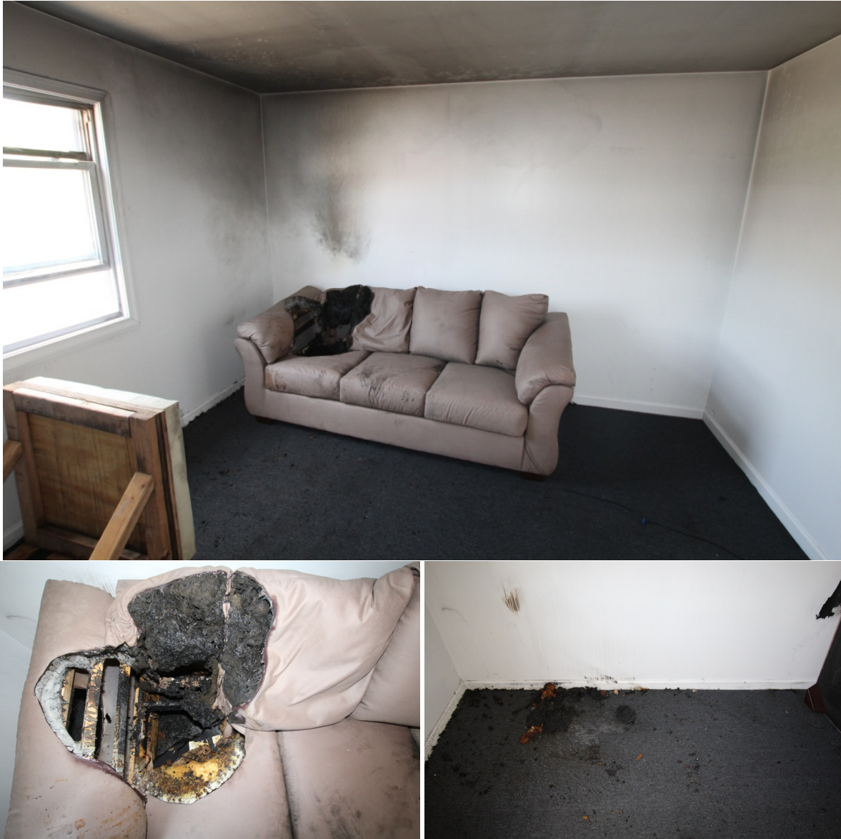
Figure 3.15: Post-test pictures of the fire room in Experiment 5.
